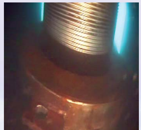
Rudder nut ready for installation onto the rudder stock.
