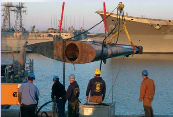
Rudder lifted from the pier using a three point lift.
