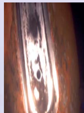
Cleaned rudder stock keyway with sheared fasteners removed.
